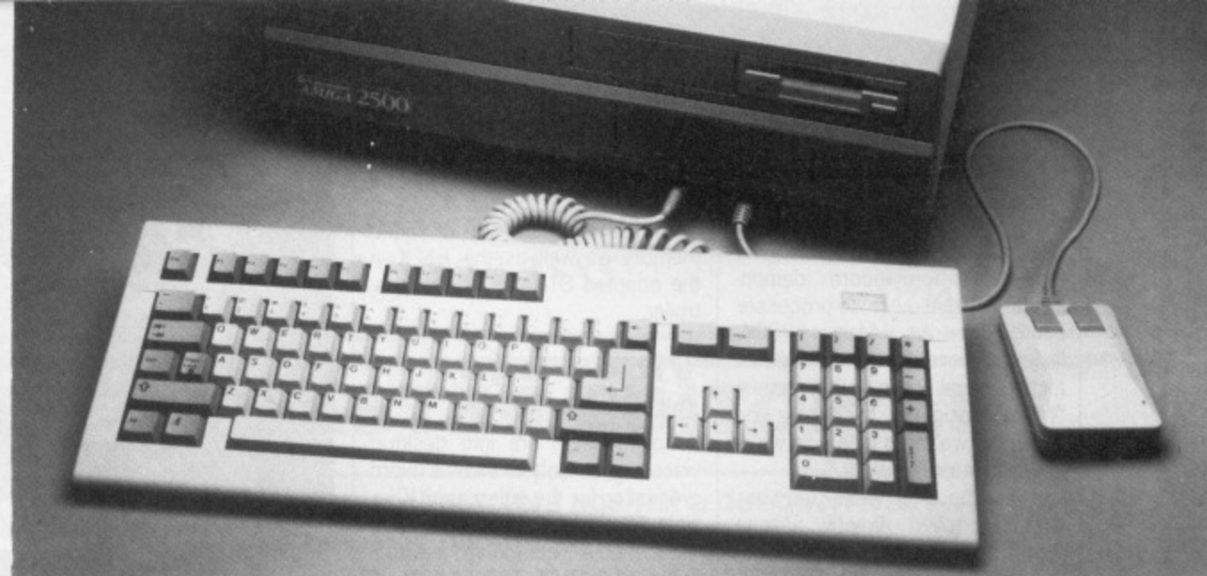
■ The Amiga 2500 – 68020, 2Mb RAM, 68881 maths co-processor. A power user's machine at $4699.
