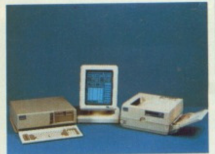
■ A typical professional DTP system, less scanner, but including an A4 monitor.
