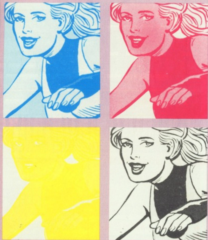
■ Any colour picture in Format is made up from four films, supplying the cyan, magenta, yellow and black components of the image.
